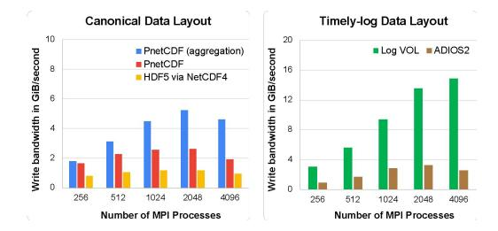
Write bandwidths of WRF evaluated on Cori supercomputer at NERSC. When output data is stored in the canonical layout, the PnetCDF aggregation strategy effectively improved the I/O performance. When output data is stored in the log layout, the HDF5 Log VOL outperformed ADIOS.
